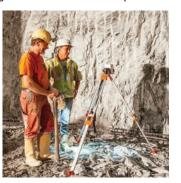
receive objective comprehensive information about geometry, condition and quality of the tunnel construction work and during all construction phases. The dibit tunnel scanner system is highly capable of complete or partial documentation or to be used for quality supervision of new tunnel construction.
